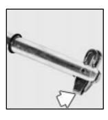
4. Push the clip so it locks in place. Pin is shown off of the vehicle for clarity.
